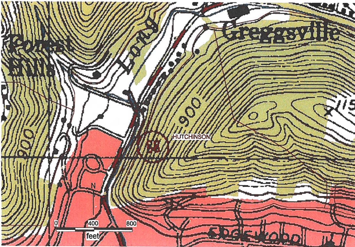
Figure 2. Close-up of the reserve boundary of the Hutchinson Mine in relation to the west end of the ridge bounded by Woodsdale and Waddles Run. Note that the reserve boundary corresponds approximately to the 770 feet above sea level (fasl) contour line.
