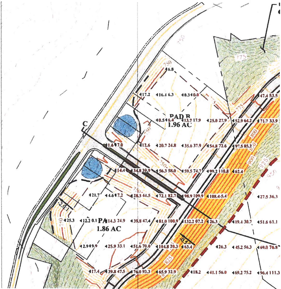
Figure 1. Close-up view of the site of Pads A and B, Phase 1 plan, as shown on Applicant's Map #29 titled "Grading Plan (Cross Sections A, B & C) note water mitigate & eng. Slope 2%," showing elevation contours in feet above sea level (fasl). Note that yellow shading represents material removed to create a highwall face.
